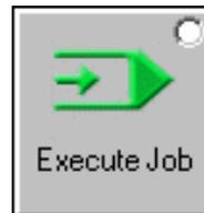
Before starting the job, go to the Execute Job mode. Press the start button on the speed throttle to start spreading.
