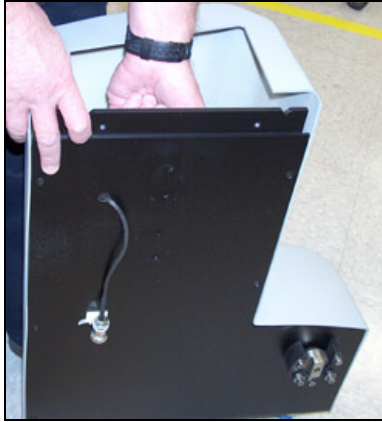
Figure 7. Right Side Column removed and balanced
