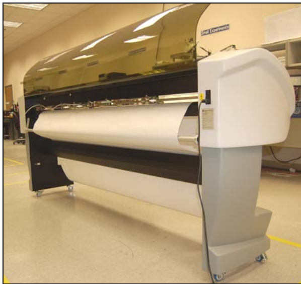
Figure 18. Paper fed through the Nip Bar and Pinch Rollers
