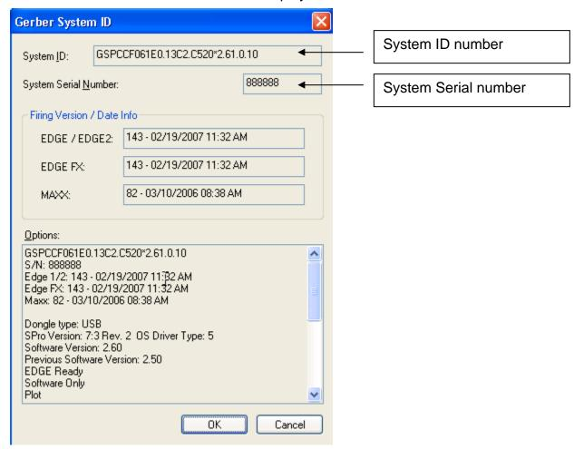
Verify the serial number displayed with the serial number printed on the label on the security key.
