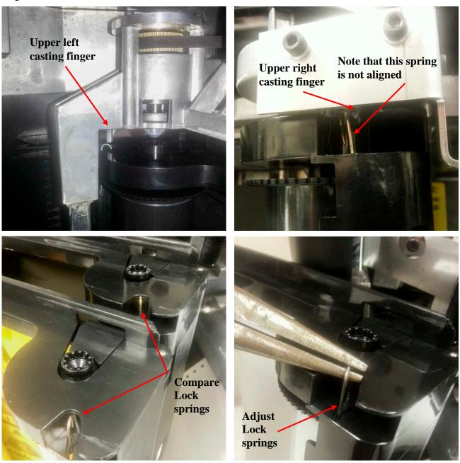
1b. Remove lock springs (pull out with needle-nose pliers) see image 1b below.
