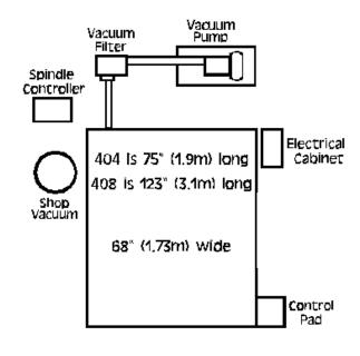
Plan extra room for storing materials and supplies, and if you intend on doing long pull through jobs. Locate the power receptacles and air supply to the right of the Sabre™. Run the wires to the optional vacuum blower motor control panel so that it can be placed near the keyboard at the front of the system.
