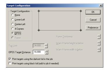
OPOS Target Distance defaults to printing additional sets of targets every 16 inches in the X length. This is recommended to ensure the most accurate cut.
