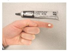
Place a pea-sized dab of lubricant onto the mid-point of the visible portion of the lead screw and work into threads. The lead screw is visible behind the print head. Avoid contact with other parts or surfaces.
