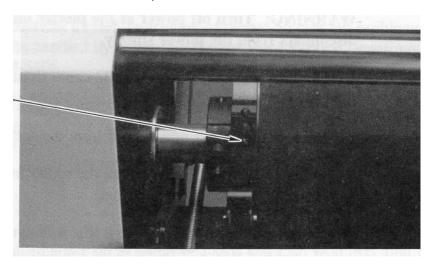
3. Also clean and oil the sliding sprocket end of the drum shaft and both sliding bail arm screws. Do not oil excessively.
