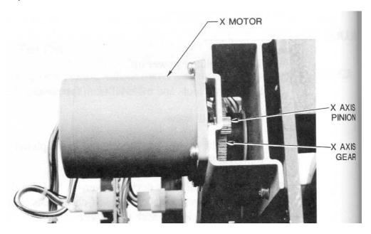
7. If the X motor pinion remains stationary (i.e., if there is backlash), locate the X motor mounting screws (Phillips head screws) which hold the X motor against the motor bracket on the side plate. Loosen these screws.
