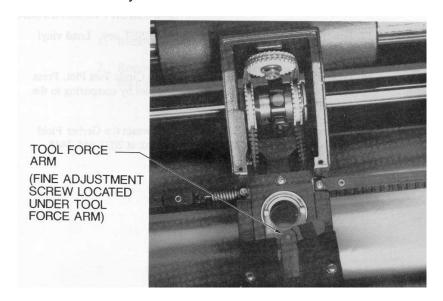
10. Raise or lower the lifter fork by turning the fine adjustment screw until the top of the lift fork is approximately 17/64" (6.7 mm) from the spindle assembly.
