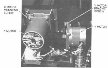
8. Apply light pressure to the motor to tighten the mesh of the X axis gear and the X motor pinion.
