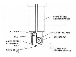
2. Turn the eccentric nut by hand, or use a small wrench, to expose more or less of the knife tip.
