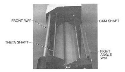
2. Apply a light coat of oil with a lint-free cloth to the front way, cam shaft, right angle way, and theta shaft.
