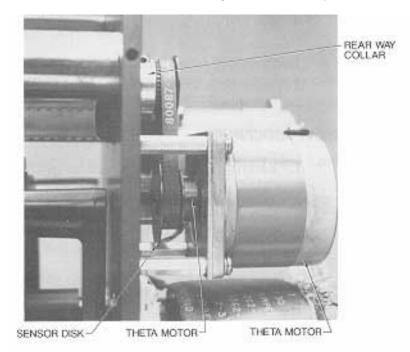
4. Then hold the RESET key down and turn on the plotter power. Access the Theta Axis Lock diagnostic by pressing the down arrow key. This locks the theta axis.
