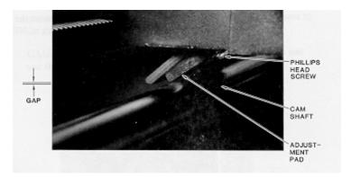
**15** Loosen the screw in the center of the adjustment pad with a Phillips head screwdriver.
